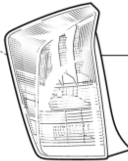
REAR COMBINATION LIGHT ASSEMBLY
